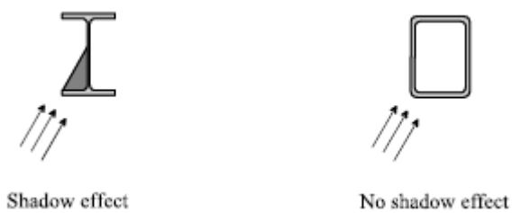
Figure 25. Influence of shape on the shadow effect.
