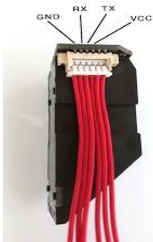
Figure 4. Pin configuration of DY50.
