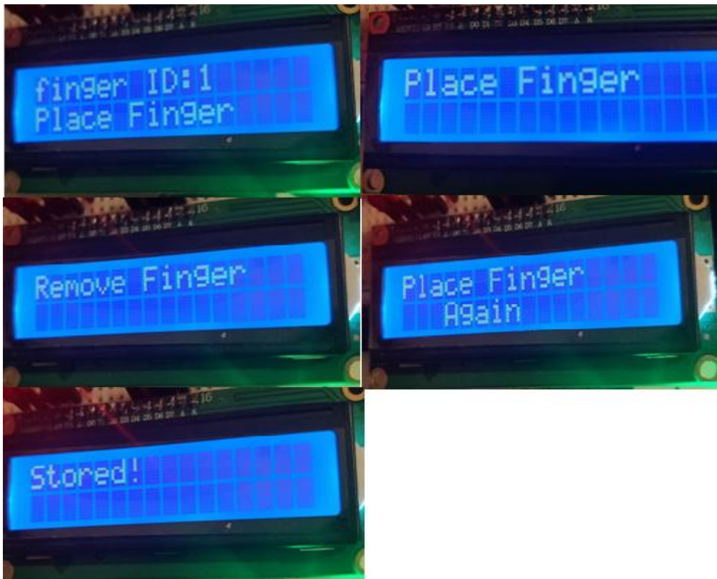
Figure 19. Messages shown in LCD during enrolment process.
