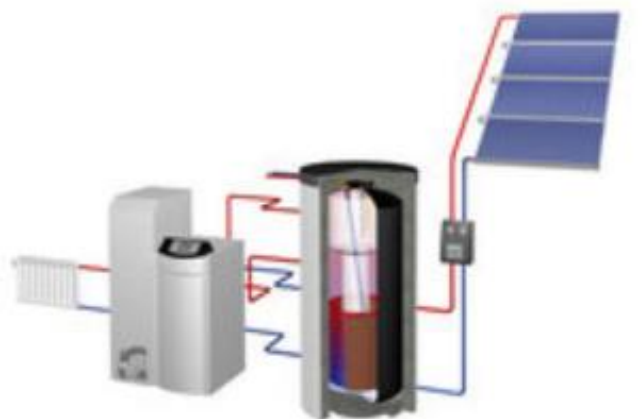
Figure 11. The structure of the hybrid solar system provided by the Ympäristöenergia company
