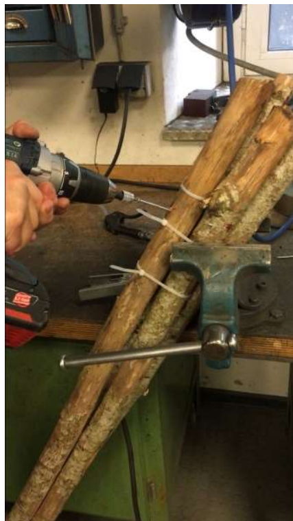
Figure 27. Power drill and screw for connecting the members
