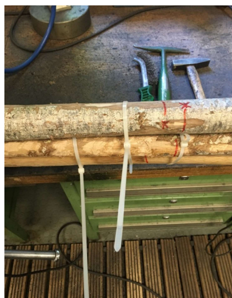
Figure 25. Temporary connection using plastic cable tie
