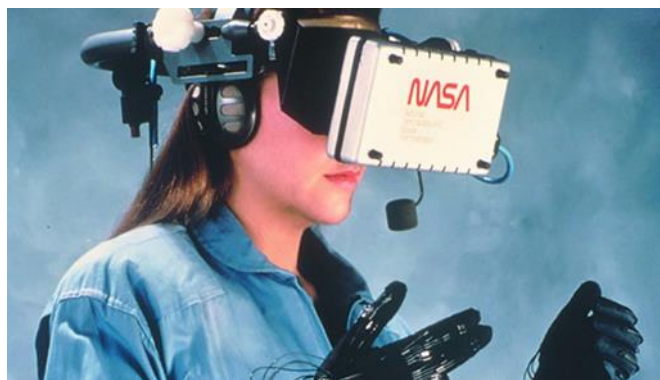
Figure 6: The Virtual Interface Environment Workstation (VIEW) developed by NASA. Source: (NASA, 2018)
