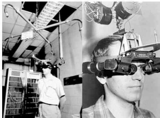
Figure 3: Ivan Sutherland's first VR headset, The Sword of Damocles. Source: (Ismail & S. Pillai)
