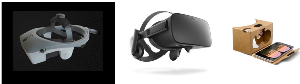
Figure 11: From left: nVisor SX60, HMD, Oculus Rift HMD, and Google Cardboard. Source: (Engadget, 2017) (Oculus, 2019), and (Google , 2019)
