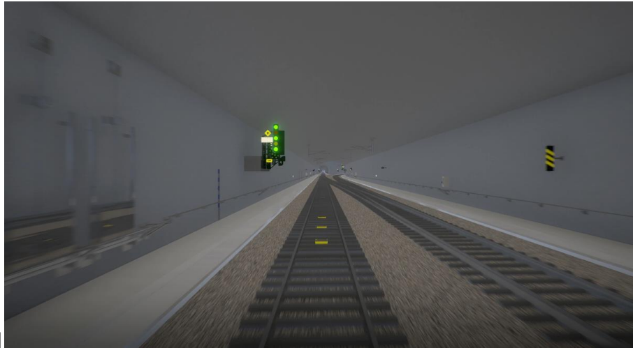
Figure 19: Train driver gave advice for moving the signal for achieving better visibility. Source: (Autodesk, 2018)
