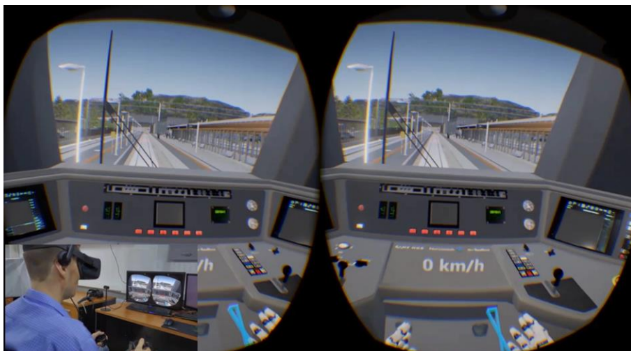
Figure 18: Train operators drive the train in VE; Real terrain mixed with the model using 3D laser scanning. Source: (Autodesk, 2018)
