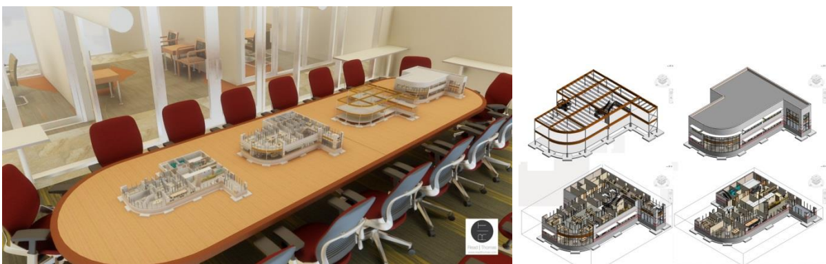
Figure 14: The left picture shows the virtual meeting room and scaled models above the table. The right picture shows multiple views for the model (architecture, structure, and sections). Source: (Read, 2017)
