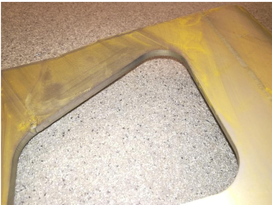
Picture 5.2. Lightening hole of Sample 3 after etching of zinc layer.
