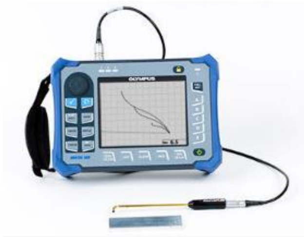
Picture 5. Portable Eddy current inspection equipment and probe [Equipment in ENSPL].
