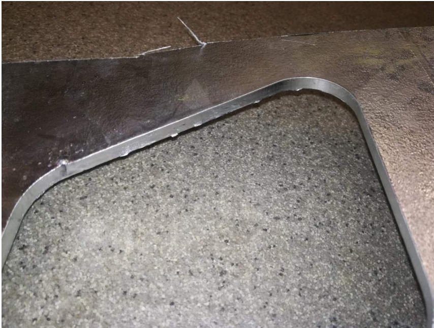
Picture 5.1. Lightening hole of Sample 3 before etching of zinc layer.
