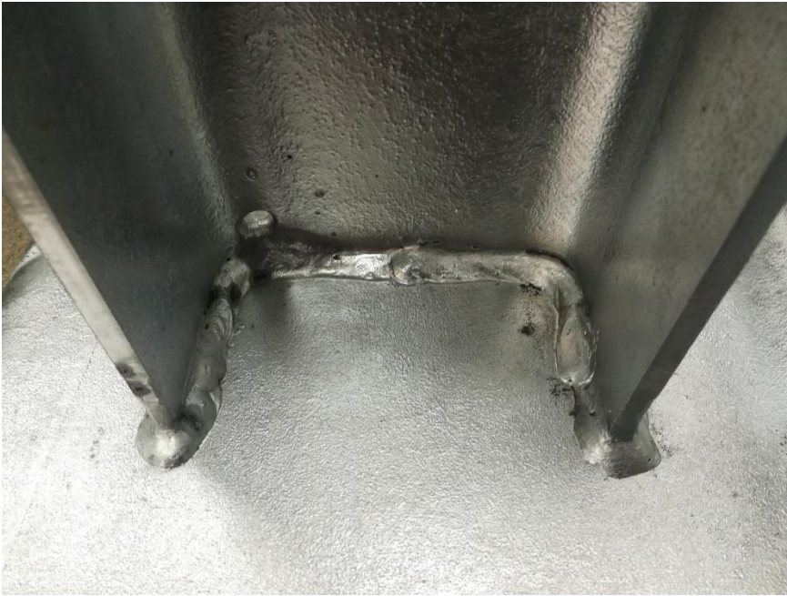
Picture 5.5. Weld of Sample 3 before etching of zinc layer.
