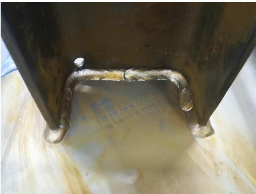
Picture 5.6. Weld of Sample 3 after etching of zinc layer.
