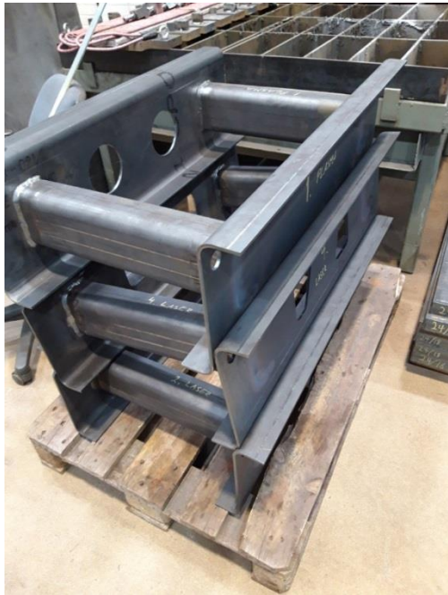
Picture 12. Composed steel structures after welding and cutting.
