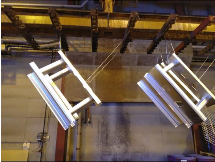
Picture 15. Sample structures suspended for hot-dip galvanization.
