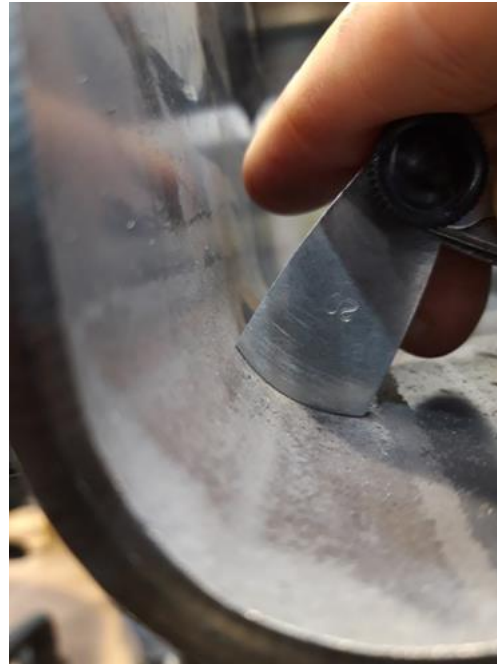
Picture 13. Confirmation of rolling radius of 20 mm with press.
