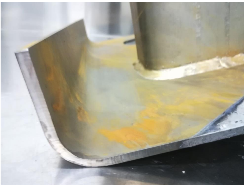
Picture 5.4. Bend of Sample 3 after etching of zinc layer.
