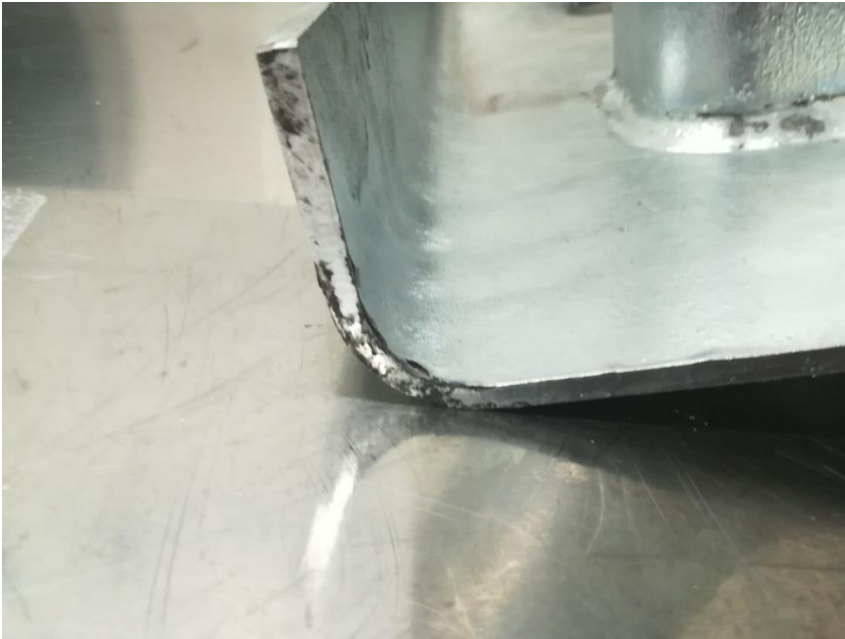
Picture 5.3. Bend of Sample 3 before etching of zinc layer.
