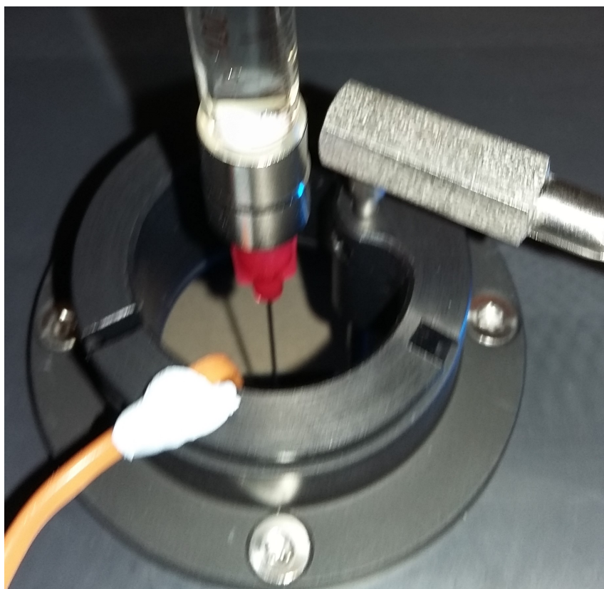
PICTURE 12. Bluetack®-immobilization of thermocouple
