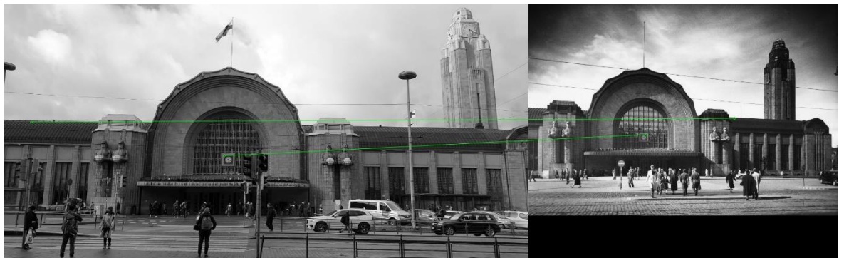
Figure 40 Matching points with SIFT (Helsinki Train Station)
