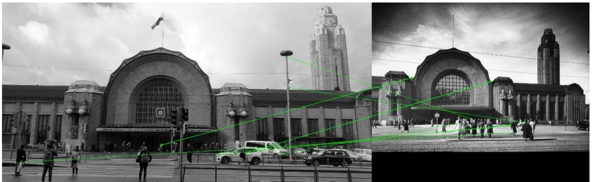
Figure 37 Matching points with ORB (Helsinki Train Station)
