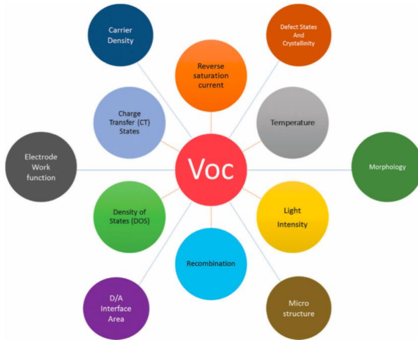
Figure 7. Factors that affect the open circuit voltage.[22]
