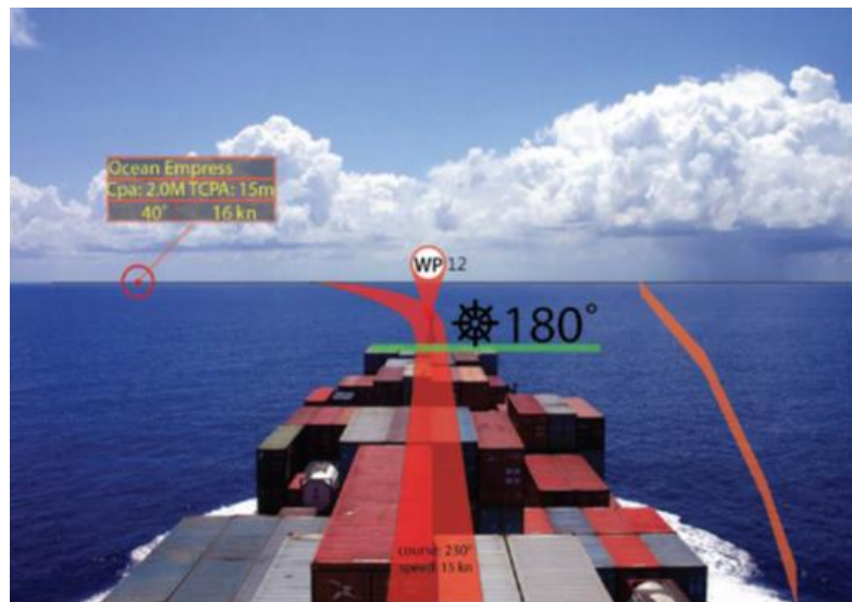
Figure 9: Example of final outside view through AR projections (de Vlaming, et al., 2013).
