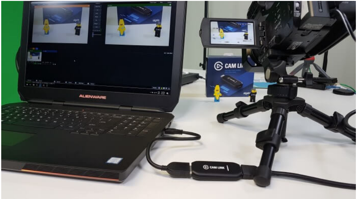
Figure 4. A camera connected to a broadcasting computer via a capture card (Image by vMix Blog)
