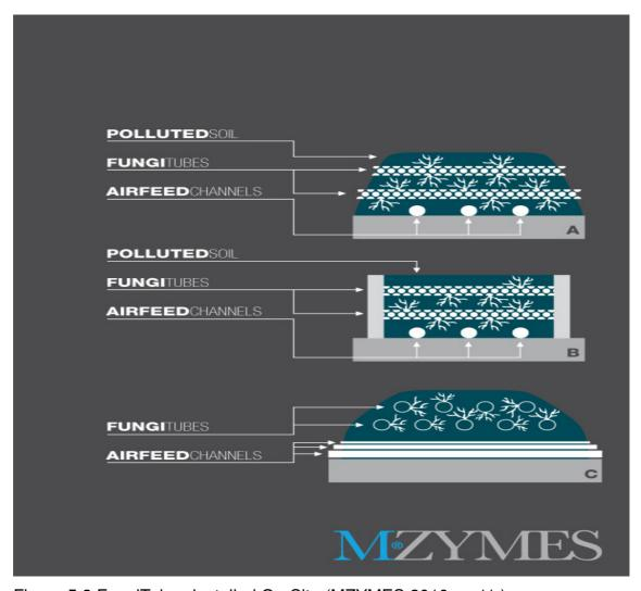
Figure 5.2 FungiTubes installed On-Site (MZYMES 2010, p. 11.)
