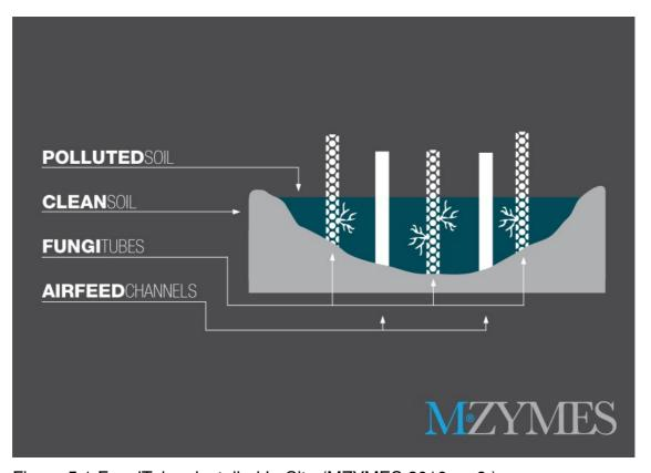
Figure 5.1 FungiTubes installed In-Situ (MZYMES 2010, p. 9.)
