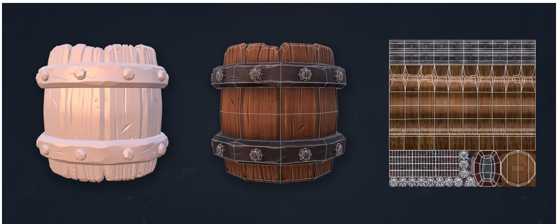
PICTURE 3. A model (left), the model's UV edges (middle), and the model unfolded into UVs on a texture image (right) (Sus 2018).
