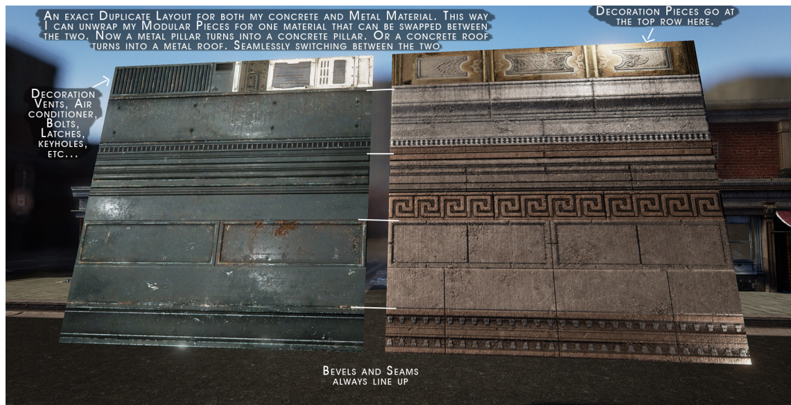
PICTURE 24. These two trim sheets are laid out identically and can be swapped between models without changing the model or UV map (Norris 2015).
