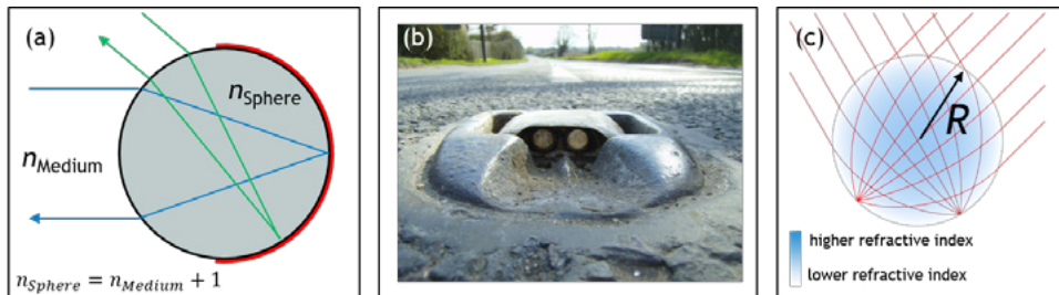
Fig. 3.3: Spherical retroreflectors. (a) A sketch of a spherical reflector (with two light rays in blue and green) consisting of a refractive transparent sphere (gray) combined with a reflective surface (red). Adapted from [20] (b) Cat's eye pavement marker. [20] (c) Optical path in a Luneburg lens. The gradient in the refractive index n is sketched in blue and increases from the surface to the center. [27]
