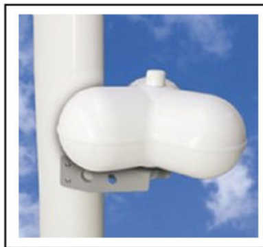
Fig. 4.11: Tri-Lens Luneburg reflector on a yacht mast. Image: The Rigging Company .
