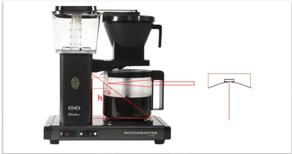
Figure 1. The distance sensor placed under the angle method
