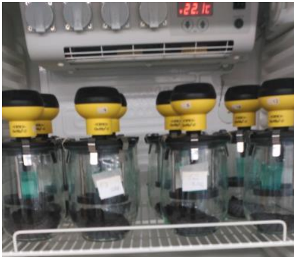
PICTURE 3.3.2 Oxitop® device inside the isothermal chamber (Photo: Luis Martín Rubio 2017)
