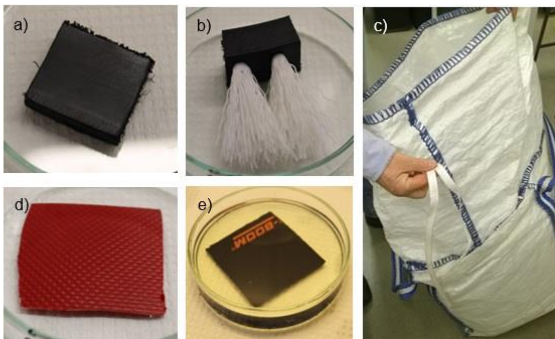
PICTURE 4. Materials used in the damage tests: a) storage tank by KK-Module Oy b) skimmer brush by Meritaito Oy c) storage bag by Knorring Oy Ab d) oil boom by Lamor Oy e) open-water boom by the Finnish Environment Institute.
