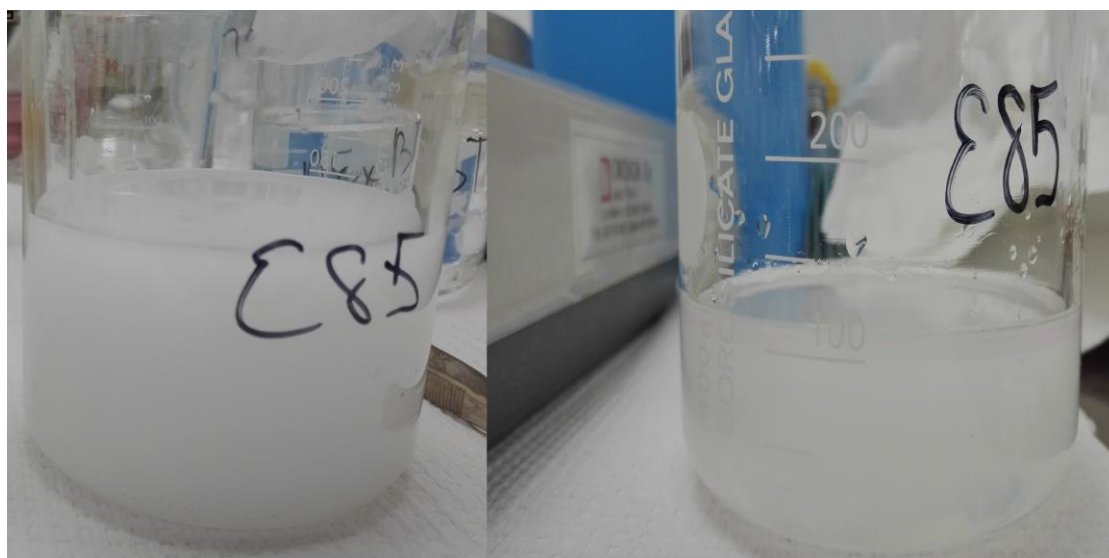
PICTURE 6. Right – E85 is added quickly and stirred. Left – slowly without stirring.
