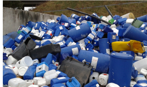
Figure 1. If plastic is collected in a proper way and it is clean, recycling will be very easy. These containers are all same polyethylene grade and pure, ready-to-use material with very little effort. (photo Reijo Heikkinen)
