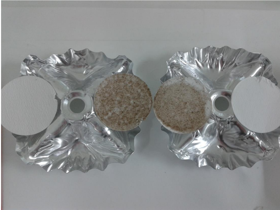
PICTURE 7. Filters before entering the oven (Paraskevopoulos, 2015)
