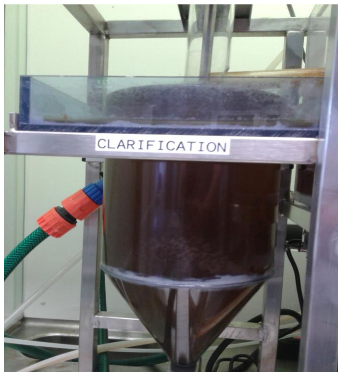
Picture 4. Clarifications chamber (Paraskevopoulos, 2015)
