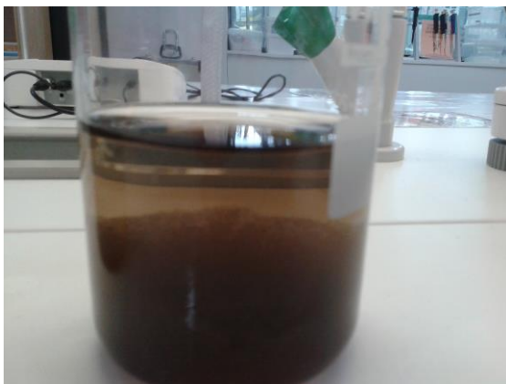
PICTURE 9. Sludge settling after 30 minutes (Paraskevopoulos, 2015)
