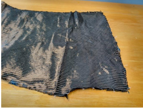
Figure 18. Carbon fiber fabric with multidirectional tows
