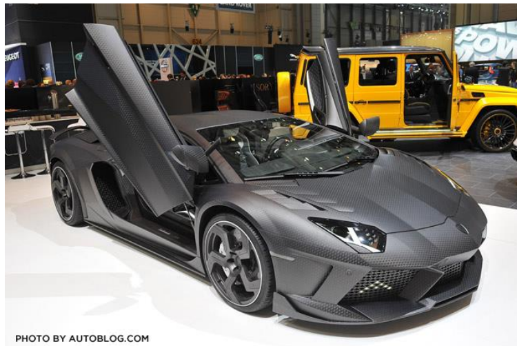
Figure 6. High-performance car in which the whole exterior is made of carbon fiber 6
