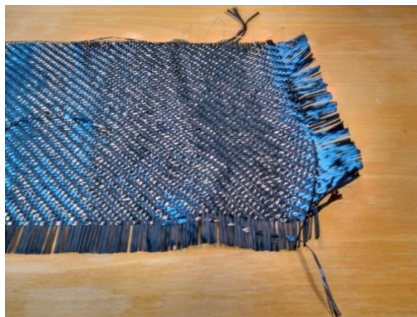
Figure 17. Carbon fiber fabric with multidirectional tows
