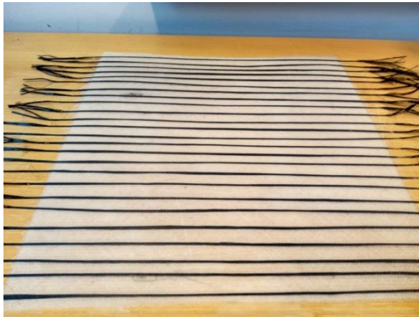
Figure 19. Carbon fiber tows held together in a resin
