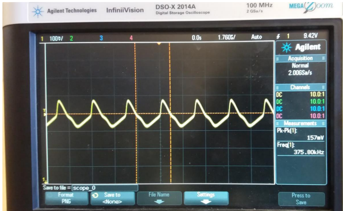
Figure 34 Oscilloscope Measurement Waveform after placing the Buffer at 0V
