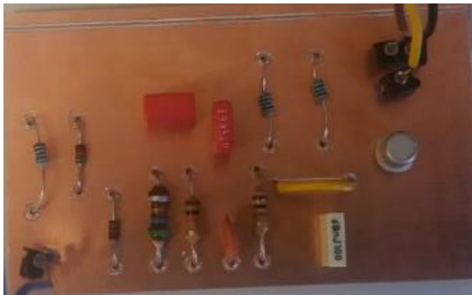
Figure 52 Milled Circuit board top side with soldered components
