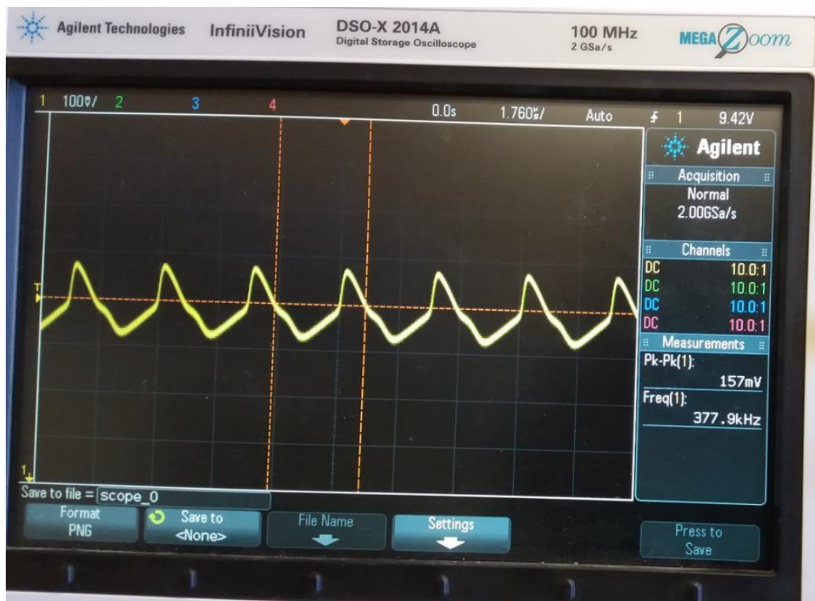
Figure 38 Oscilloscope Measurement Waveform after placing the Buffer at 2V
