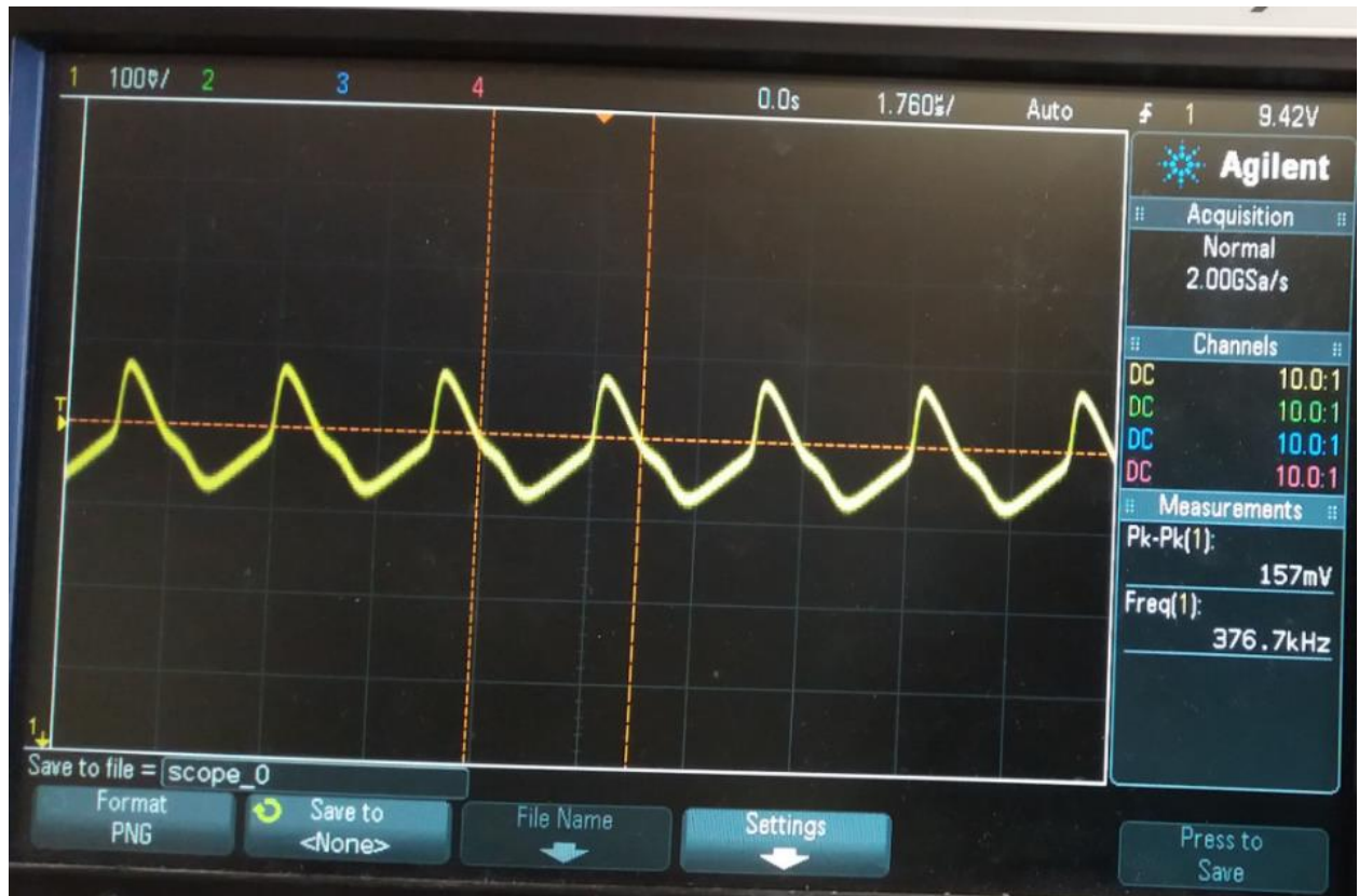
Figure 22 Oscilloscope Measurement Waveform after placing the Buffer at 1V
