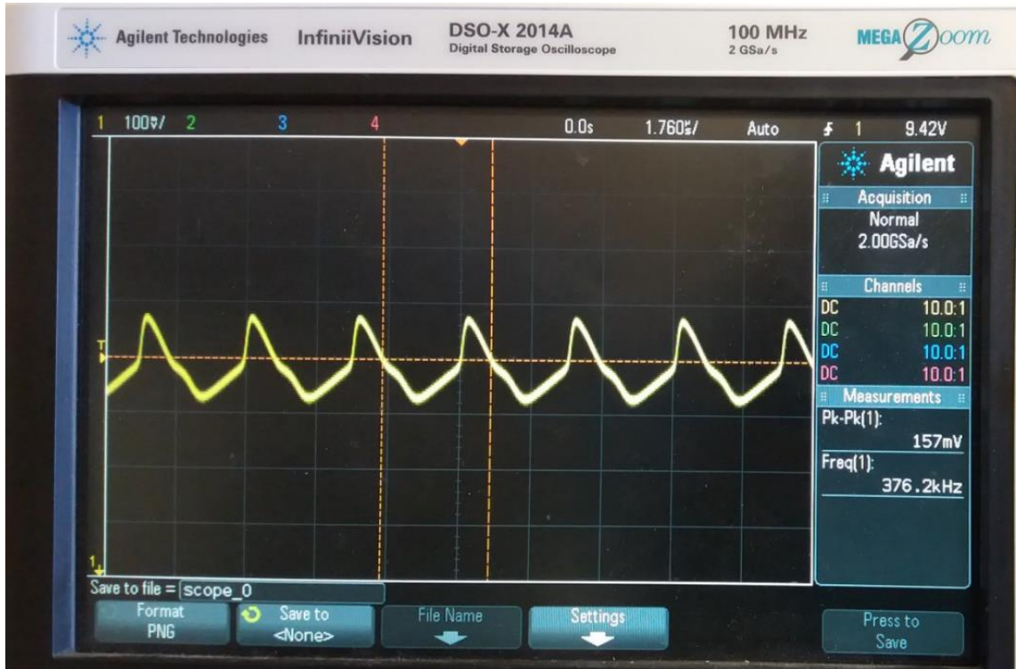
Figure 35 Oscilloscope Measurement Waveform after placing the Buffer at 0.5V
