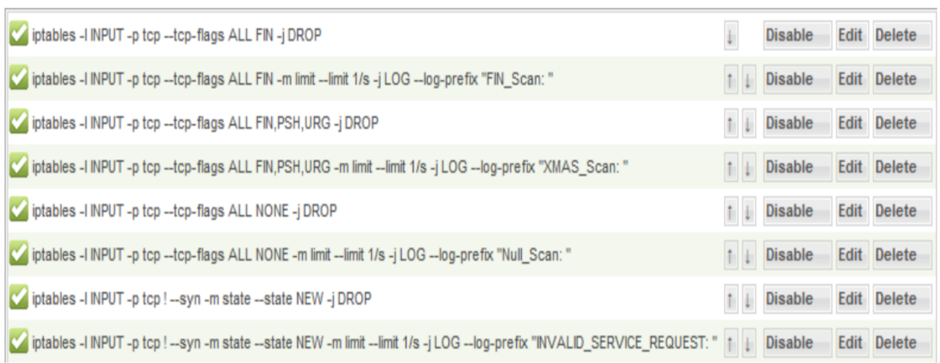
Figure 26. Rules for blocking scan port using NMap
