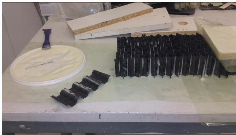
Figure 3.14. Building of the carbon fibre honeycomb core
