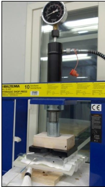
Figure 3.8. Mould under press and heating
