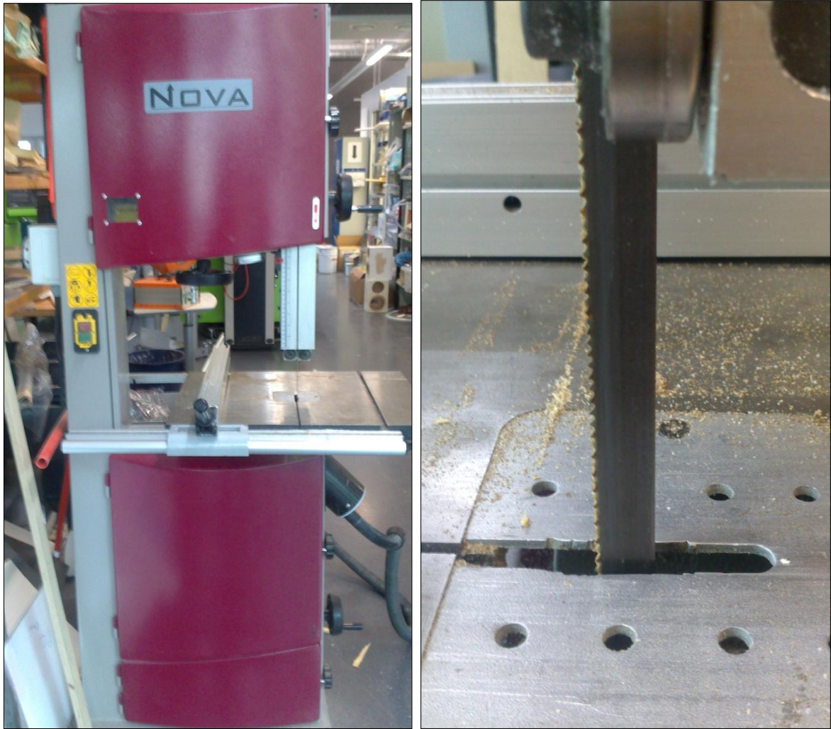
Figure 3.11. Bandsaw and the blade used for slicing of the layers
