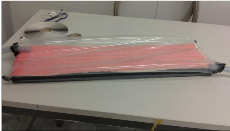
Figure 3.2. Vacuum impregnation of fibre glass with epoxy resin
