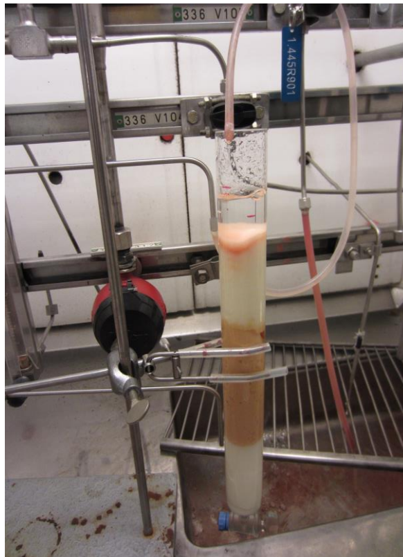
Picture 16 Enrichment test after one week, notice reddish layer, which appears because of the iron in the feed water.
