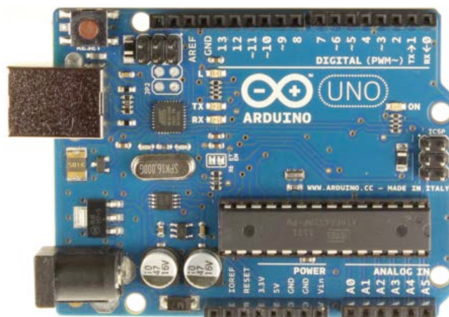
Figure 11. Arduino Uno R3 (Arduino board used for project)
