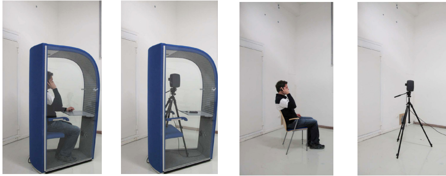
Fig. 1. Photographs of the two phases of the ISO 23351-1 test. First, the sound power level is determined for the loudspeaker placed inside the booth to the head position of a standing occupant. Loudspeaker is placed to the position of occupant's mouth (two leftmost figures). Second, the sound power level is determined for the bare loudspeaker by keeping the same position, but the booth is removed. The sound power level of the loudspeaker is constant in both measurements.
