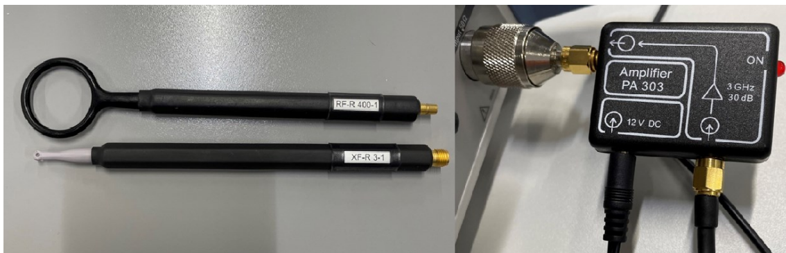
FIGURE 24. RF-R 400-1 and XF-R 3-1 H-field probes, and 30dB preamplifier where the probe was connected.
