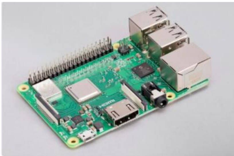
Figure 2. Raspberry Pi 3 model B+.
