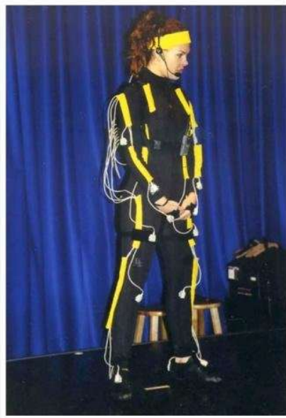
Figure 30: A performer wearing a suit for magnetic motion capture (AMM, 2010).
