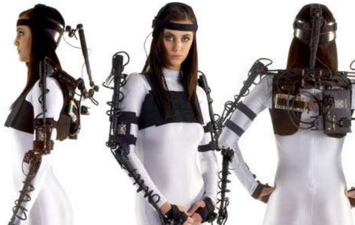
Figure 28: Gypsy Torso™ - Upper Body Mocap system (Meta Motion 2004).
