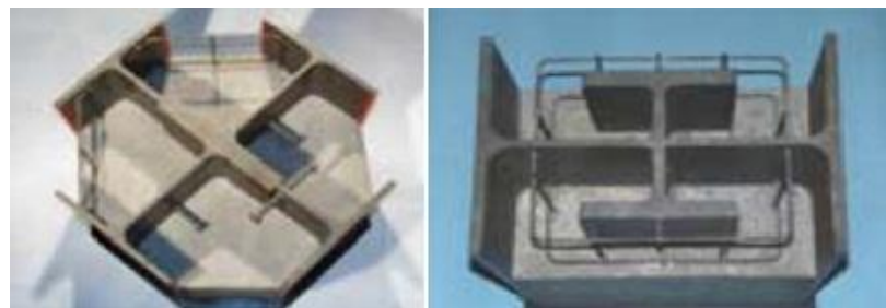
Figure 18. Partially concrete encased sections
