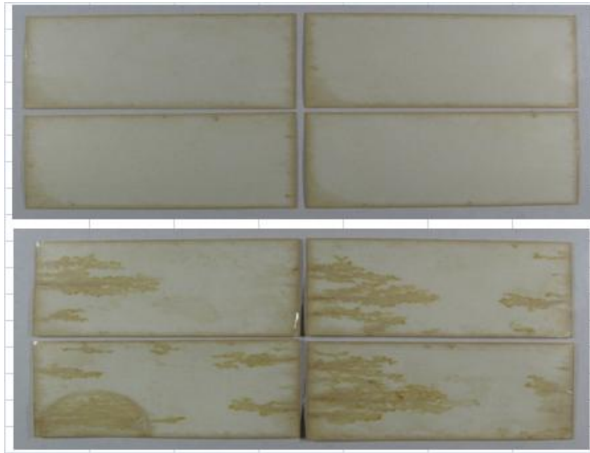
Figure 9. Effect of cutting efficiency on edge-wicking. Test strips from sharp and clean cutter (top) clearly showed less wicking compared to strips obtained from blunt cutter (bottom).
