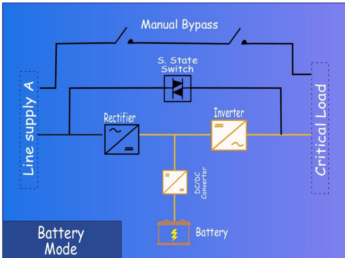
Figure 16. Battery mode during power failure or outage.
