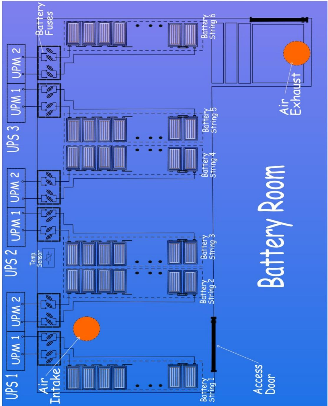
Figure 3. Battery connections scheme in the battery of DC2.
