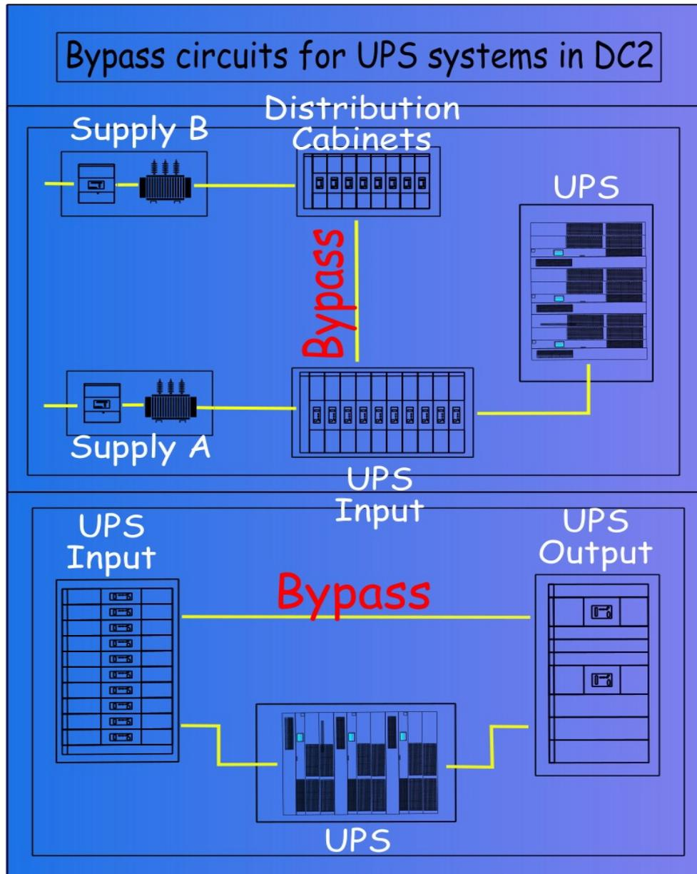
Figure 5. Bypass circuits for the UPS system. The bypass circuit on the top is used to omit the supply from transformer A. The bypass circuit on the bottom is used to omit the UPS units.
