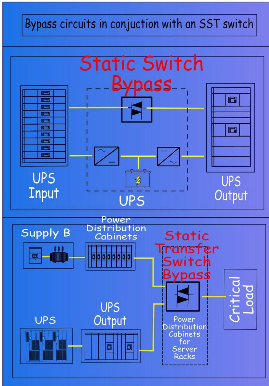
Figure 6. Bypass circuit in conjunction with SST switch. On the top box, the SST switch creates a circuit bypass the UPS units in case of UPS failure. On the bottom box, the SST switch choose between source A and B in case of line failure at PDN A or B.
