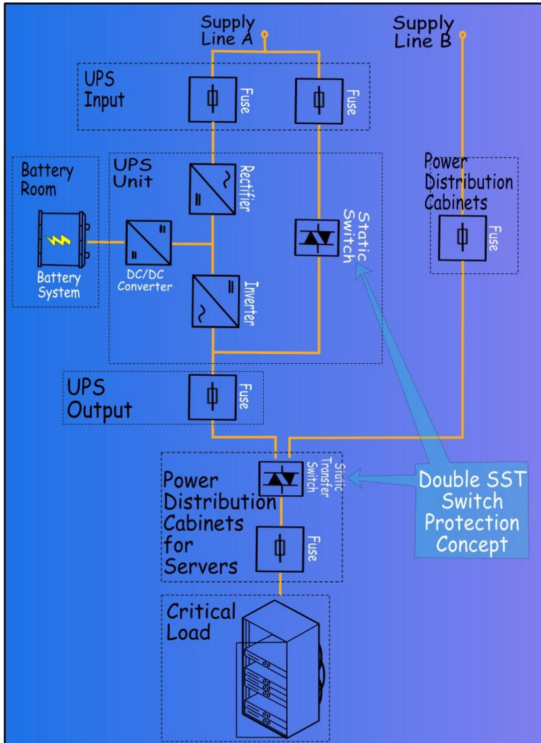
Figure 12. Double SST switch protection concept for the critical load of data centers.
