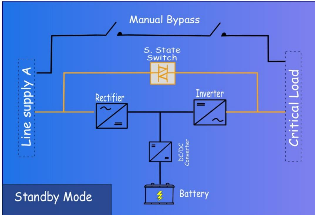
Figure 14. Power flow of Passive Standby Mode or VFD.
