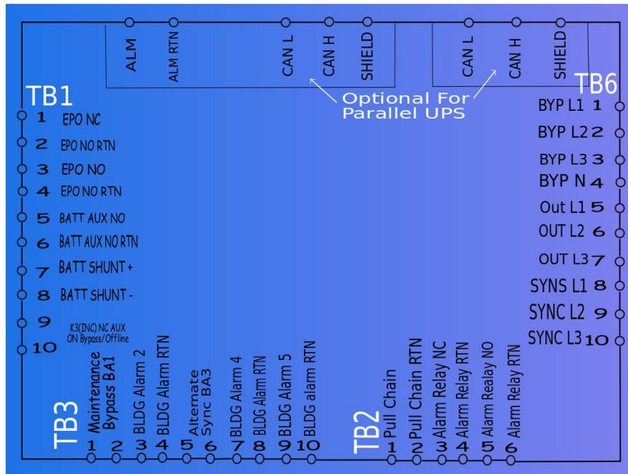
Figure 4. Control connections for the UPS units 9395P.
