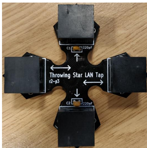
Figure 25 Ethernet LAN tapper used in the project
