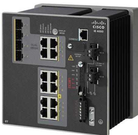
Figure 8 Cisco IE-4000-8T4G-E switch used in the thesis /14/
