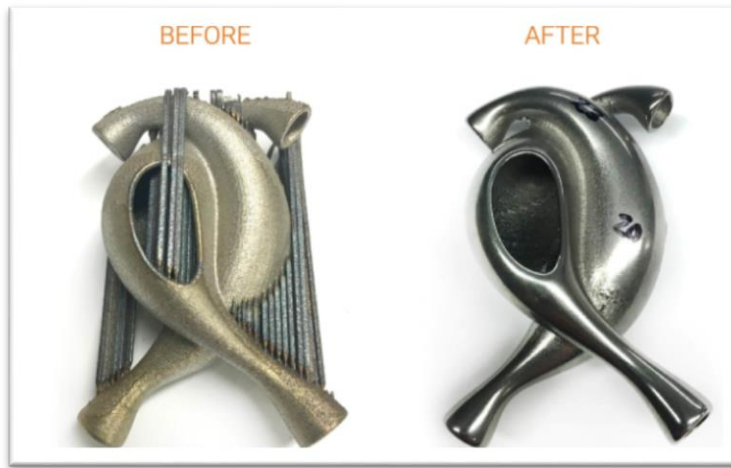
Figure 7 3D printed object in Titanium, before and after postprocess which included support structure removal and surface texture finish [14]
