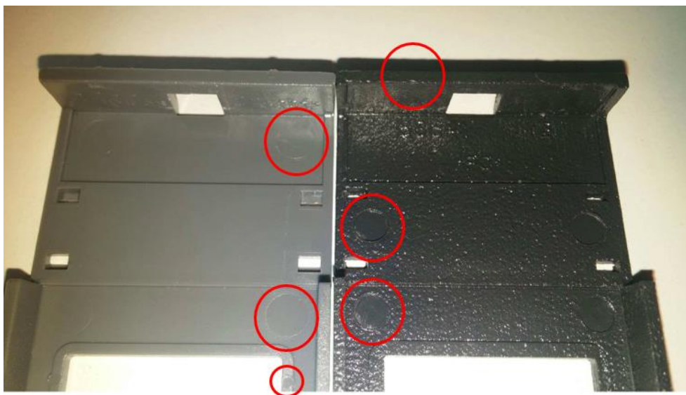
Figure 34 Circled are the marks from the ejector pins, (new cover to the right)
