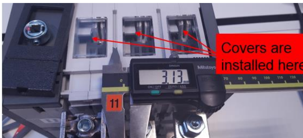
Figure 35 Cover mounting to the switch pole
