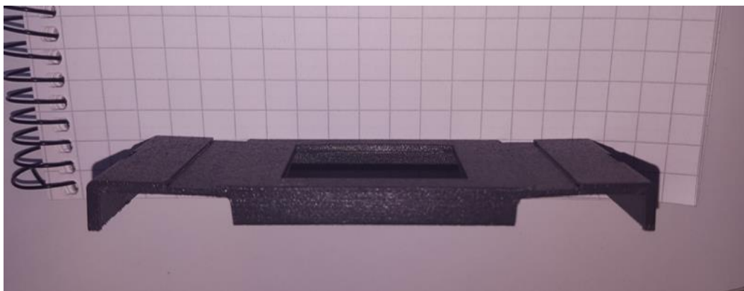
Figure 37 Unwanted curvature of the cover
