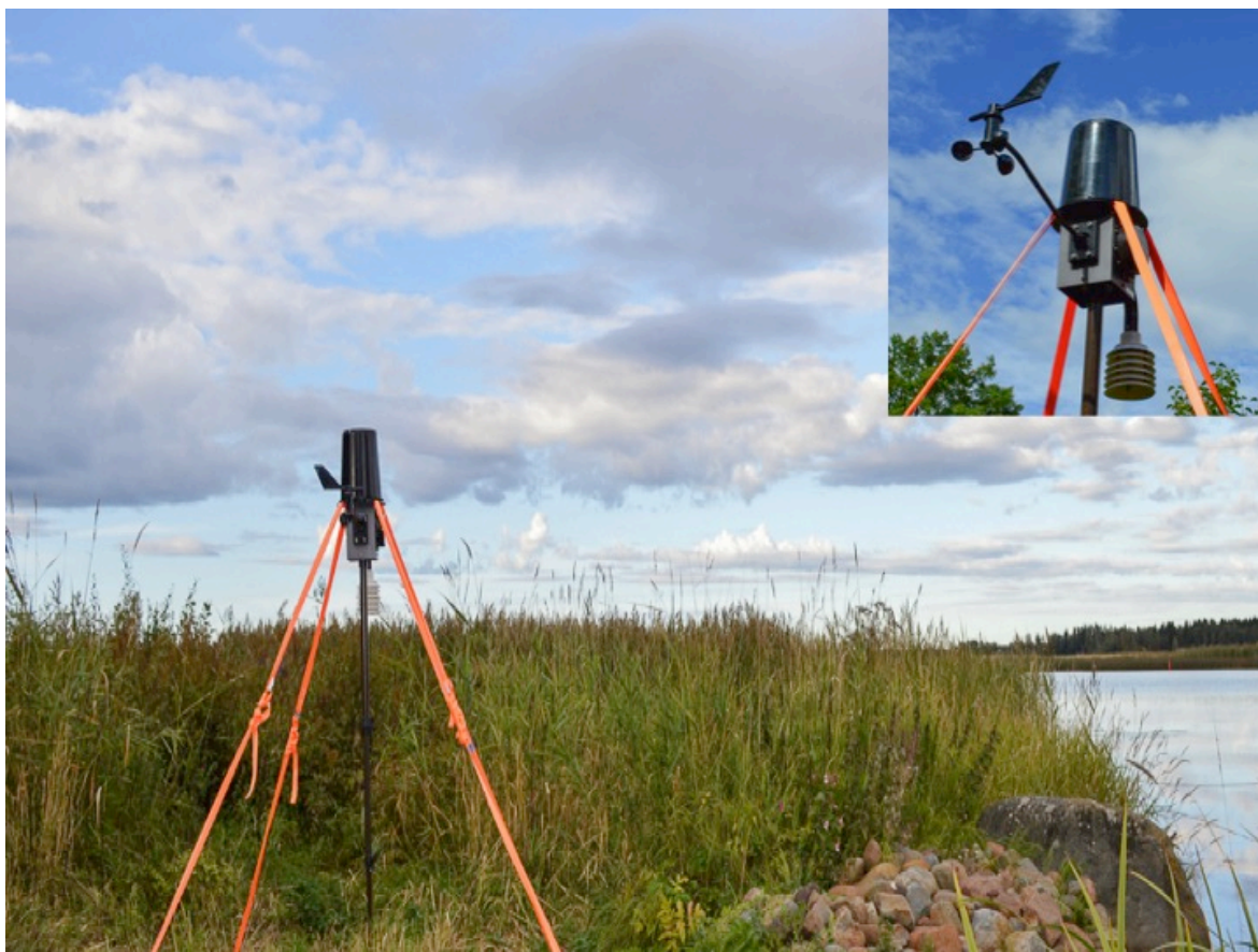
Figure 5. The weather station from the a-Lab on the site.
