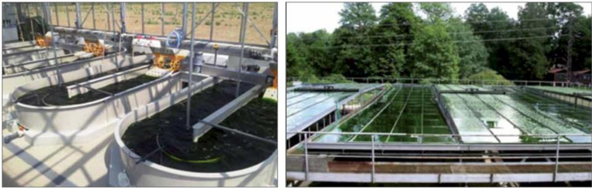
Open cultivation systems for cultivation of microalgae; left: Race way ponds; right: cascade system
