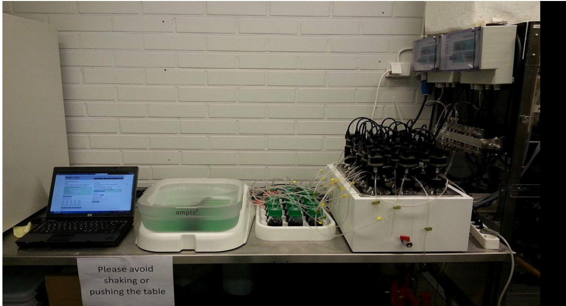
Figure 10: Ready set up for AMPTS II before start up.
