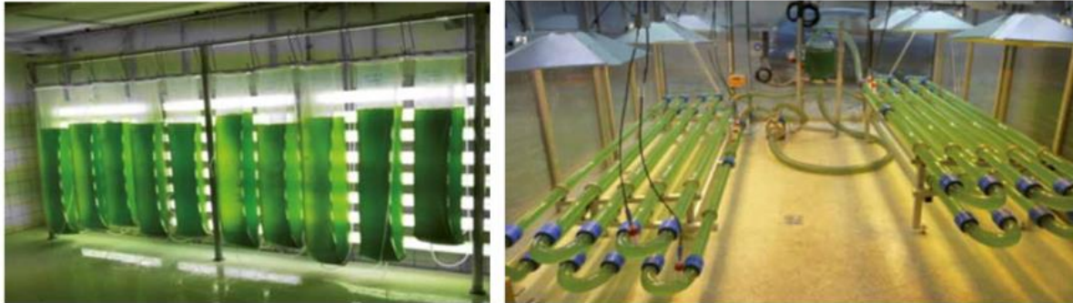
Closed cultivation systems for cultivation of microalgae; left: sleeve-bag photobioreactor; right: tubular photobioreactor
