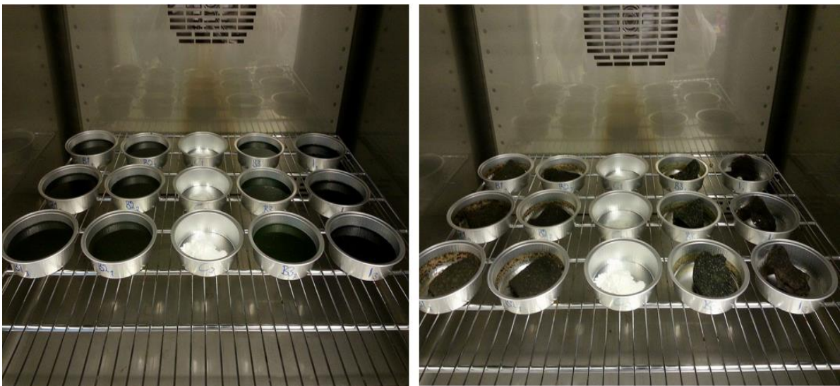
Figure 8: Samples of algae B1, B2, cellulose, Scenedesmus sp. and Inoculum from left to right respectively; left before drying and right after drying.
