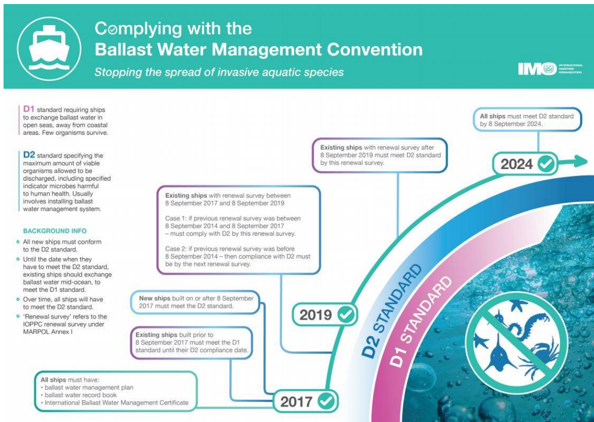
Picture 1. The implementation schedule of the BWM Convention (Implementing the Ballast Water Management Convention, n.d.)
