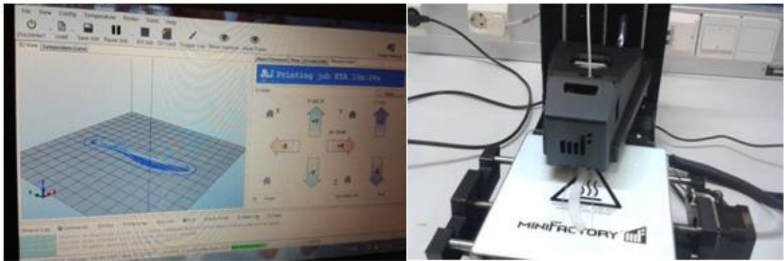
(b) Desktop image of glider's part being printed (d) Product being printed
