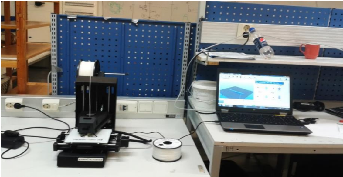
Figure 17 FDM 3D printer at Arcada lab [photo taken by- Ramji Pandey]
