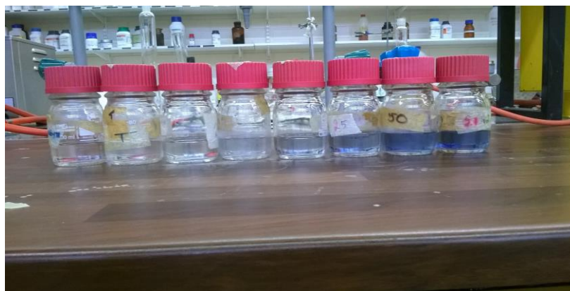
Figure 7-2 Calibration solutions before analysing with spectrophotometer
