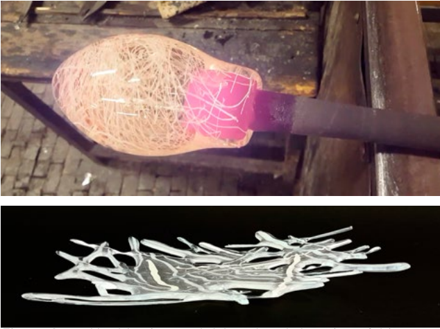
Figure 4. Hot blowing work (above) and slumping of thin canes with white core (below)
