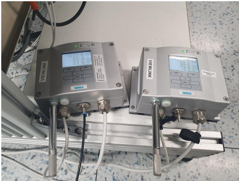
Figure 18 PTU301 devices logging ambient and chamber pressure
