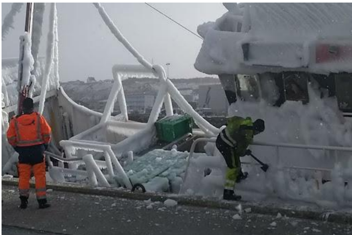
Figure 2 Vessel loses stability due to heavy icing (Team, 2018)
