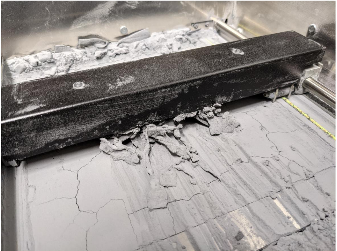
Figure 46. Recoater crash, detail shot of the recoater
