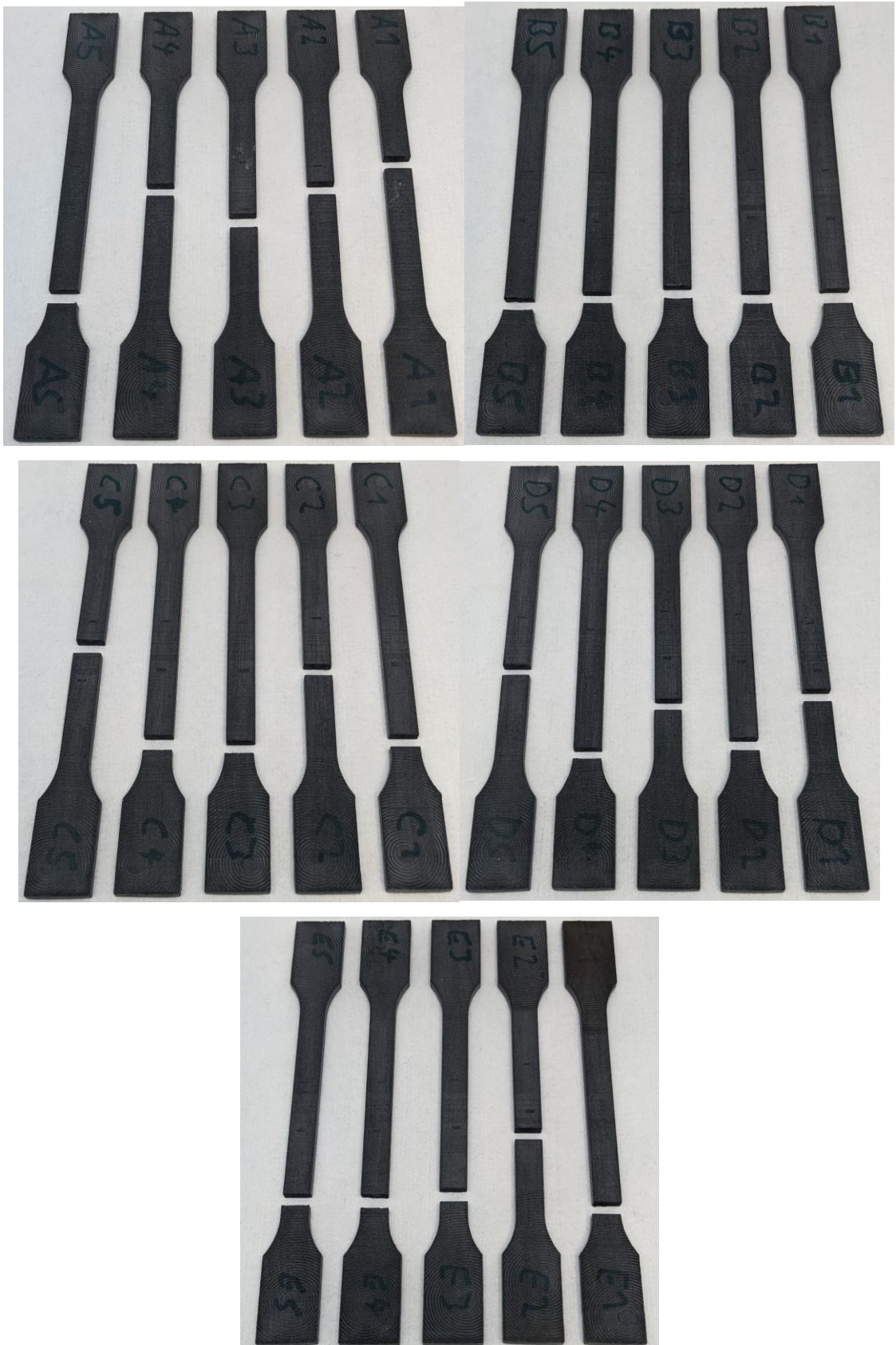
Figure 51. Illustration of fractured vertical tensile specimens V-A1 - V-E5
