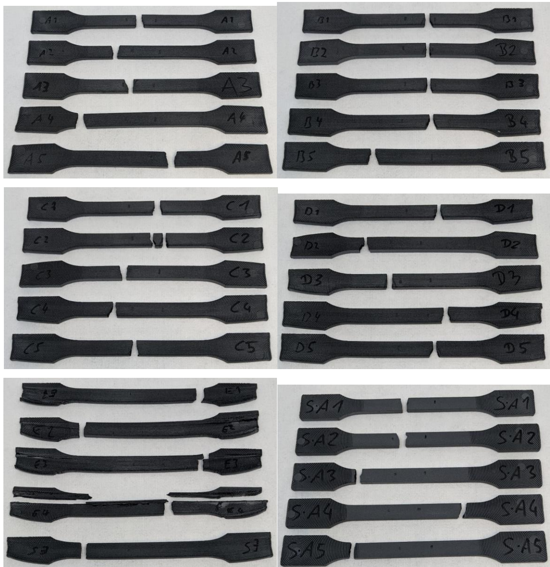
Figure 52. Illustration of fractured horizontal tensile specimens H-A1 – H-E5 and horizontal-flat tensile specimens HF-1 - HF-5
