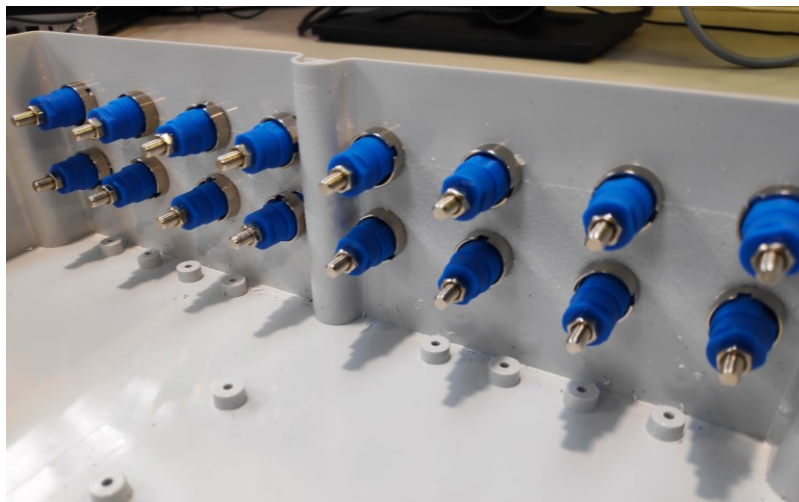
Figure 12. Enclosure with the sockets installed.
