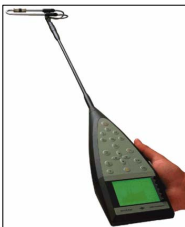
Figure 5.4. B&K 2260 with extension stem and probe /5/.
