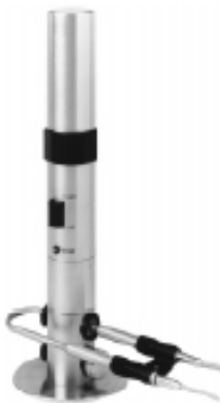
Figure 3.21. Sound pressure calibration using a pistonphone and an intensity coupler.
