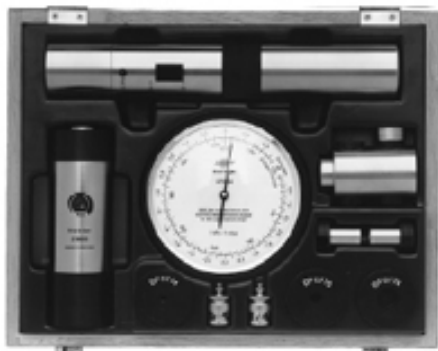
Figure 3.19. B&K Sound Intensity Calibrator Type 3541 Components in Their Case.
