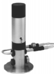
Figure 3.24. Verifying a pressure-residual intensity index.
