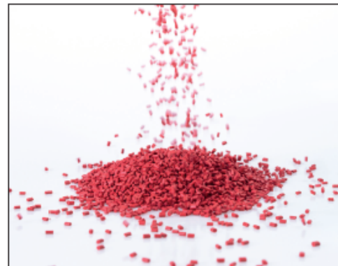
Fig. 2: Plastic granulate for injection molding or extrusion
