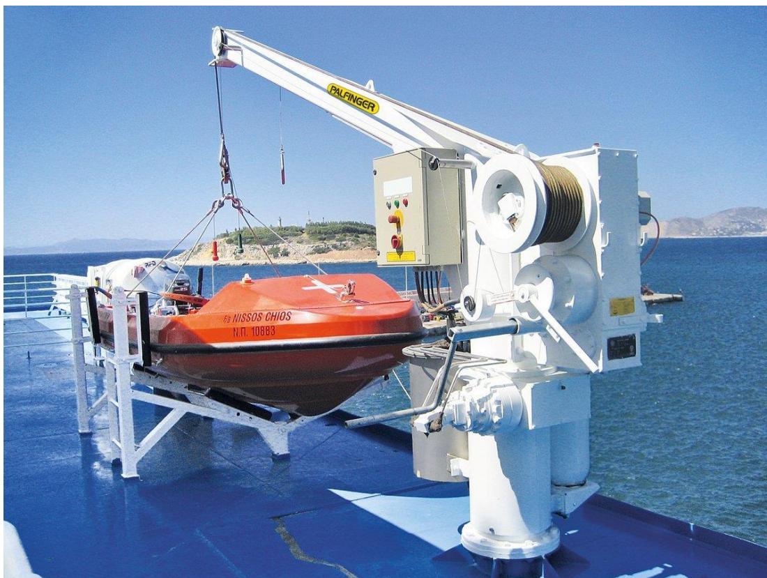
Picture 1 - Palfinger rescue boat and davit system (Palfinger Marine, w.y., a)
