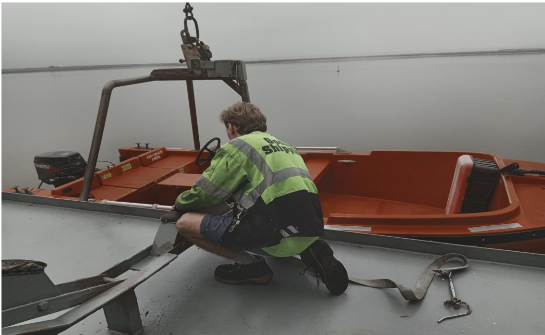
Picture 5 - Testing of launching and recovery without any persons onboard (Valtteri Rantala, 2020)
