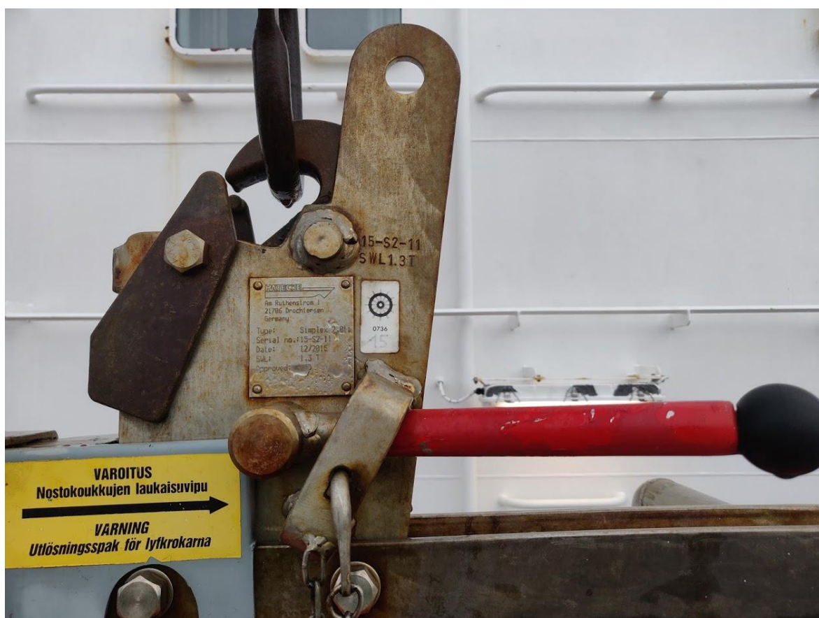
Picture 3 - Hatecke Simplex 2.0 off-load release hook is listed as compliant in GISIS (Valtteri Rantala, 2020)
