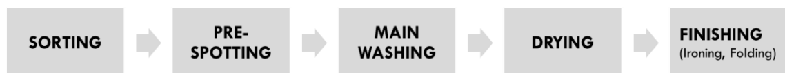
FIGURE 3. The general operation of industrial laundries (Visualisation based on information of ASEAN 2012)
