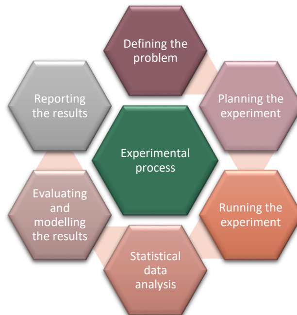
Figure 3. Framework for experimental design. The objective of the Design of Experiments (Doe) statistical tool. [12, p. 27]
