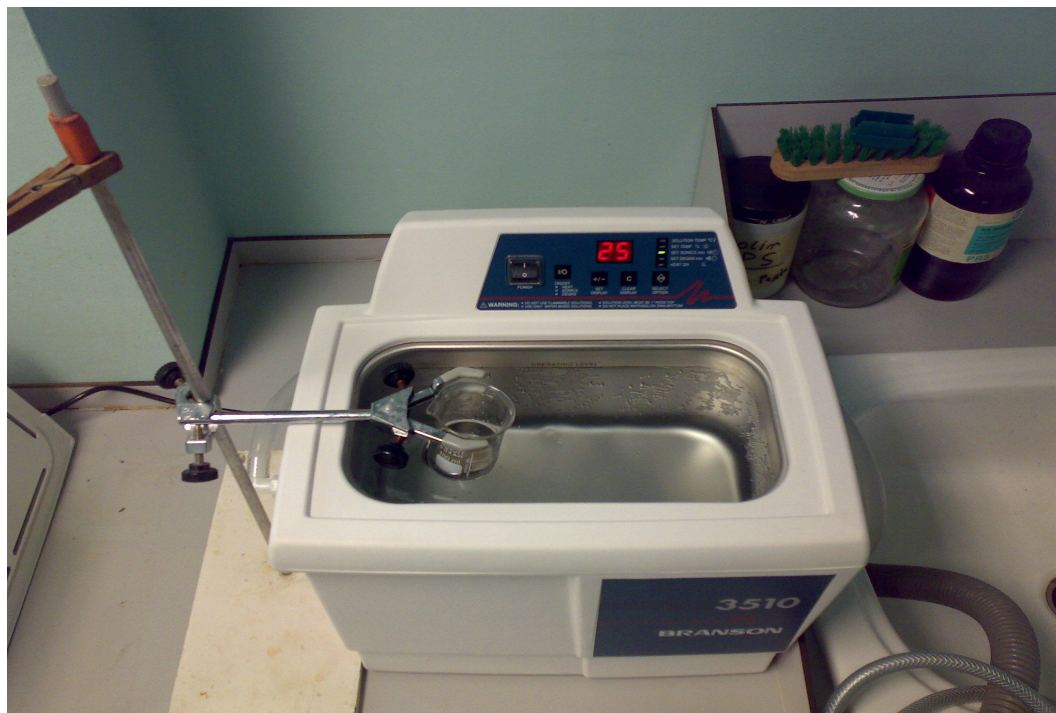
Figure 16. Epoxy/MMT in the ultrasonic bath
