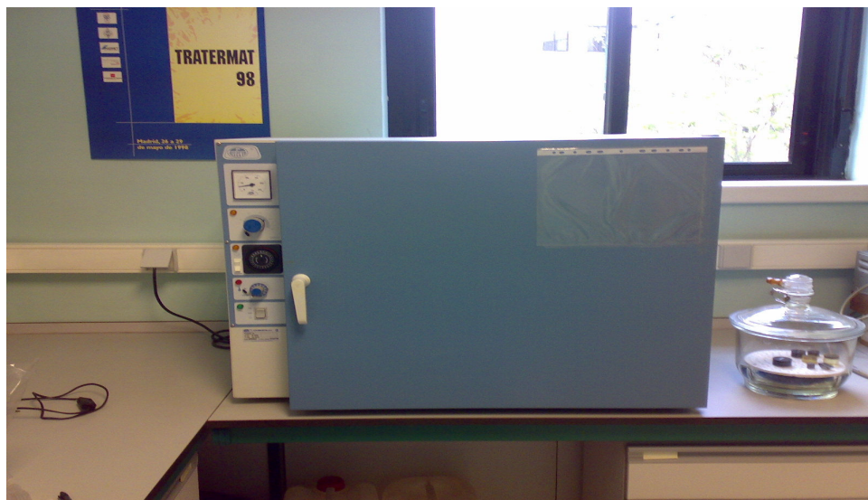
Figure 17. The Oven used for curing the composites.
