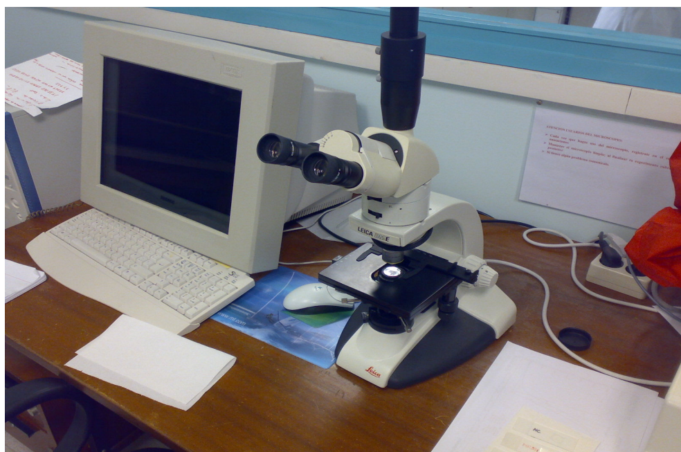
Figure 18. A Leica polarising transmission optical microscope used for monitoring the dispersion
