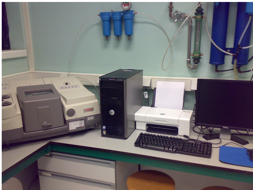
Figure 14. A Fourier transform infrared spectrometer and computer for monitoring the results.
