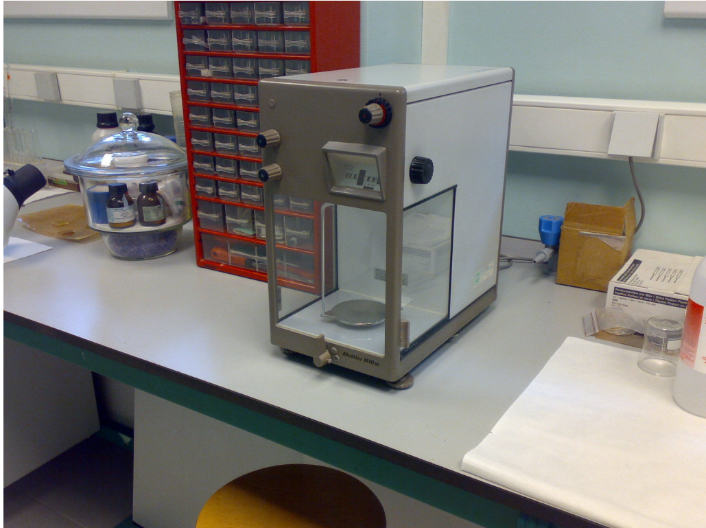
Figure15. Analytical balance used for weighing the materials
